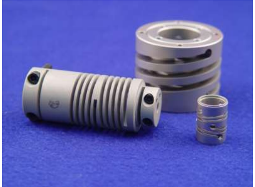
Machined Spring Flexure Configurations for Compression and Extension Springs that resist rotating given deformation
