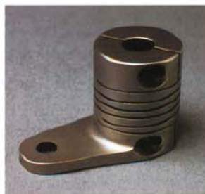
Integrating a lever arm into a clamp attachment flexure allowed linear motion to be converted to rotary motion.
