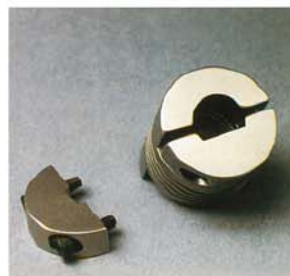
Detachable caps permit flexure installation where components cannot be spread apart to slide the flexure onto component shafts.
